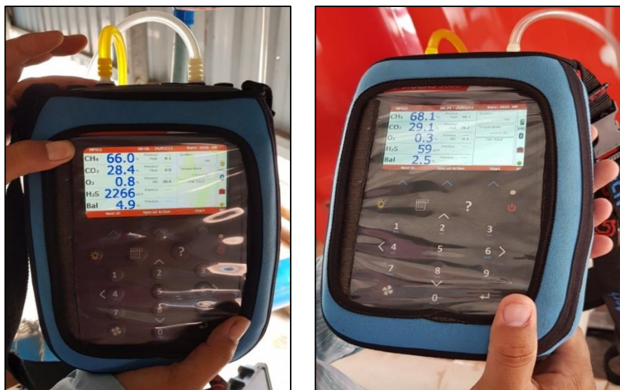
Fig. 3 Biogas quality measured before desulfurization (left) and after desulfurization (right)
